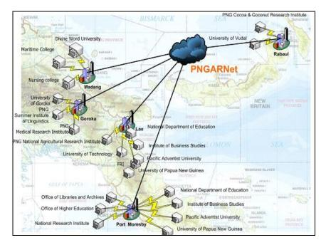
**Figure 3** Beginnings of the PNGARNet data communication network linking PNG education and research institutions. The AsiaSat 4 communications satellite provides the data communication channels between institutions as well as Internet access through a Network Operations Centre in Hong Kong.
