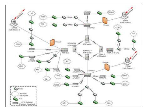
**Figure 2** A land line design proposed for ERNet in 2001 to link PNG education and research institutions and to provide bulk purchase of bandwidth for Internet access. Whilst the design was quite visionary, it was expensive and required a level of funding that was not available at the time. Presently available off-the-shelf technologies involving satellite rather that land line communication overcome many of the problems offered by this design.
