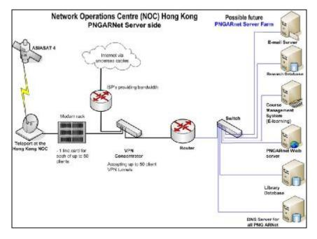
Figure 9 shows server-side equipment at the NOC in Hong Kong. Each client institution has its own VPN channel which is accepted by the VPN concentrator which can accept up to 50 channels. Each channel needs a modem to match the client side modem shown in
