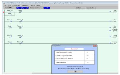
Figure 3: Red-orange – green-orange-red-orange-green simulating ladder logic diagram.
