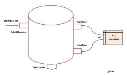
Figure 5: The PLC controlled oil storage/dispensary unit.
