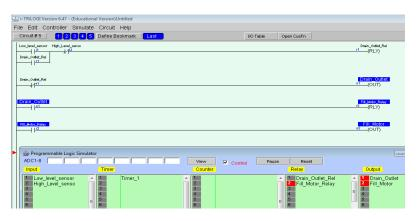
Figure 6: Simulation of coconut oil storage and dispensary facility
