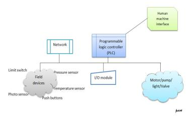
Figure 1: A generalized view of PLC design at Napanapa oil refinery, Port Moresby.
