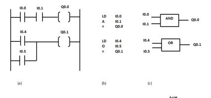
Figure 2: Programming format using Siemens PLC notation.
