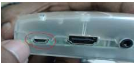
Simply plug a micro-USB power cable into the power socket of the RACHEL-Pi.
