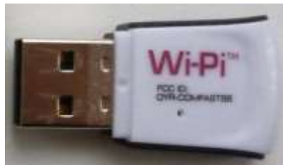
Additionally, a Wi-Pi module can be added to the Raspberry-Pi to enable connection to a Wi-Fi network. Especially for a Raspberry Pi 2.
