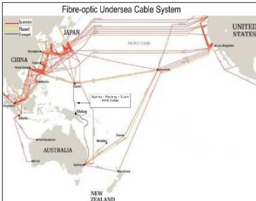
**Figure 5** Portion of the published world map of undersea cables. Note the density of cables entering and leaving Hong Kong where the Network Operations Centre (NOC) for PNGARNet is located. This will enable ISPs to provide PNGARNet users high speed access to the Internet. Shown also is the Sydney-Guam PIPE cable which has an outlet to
