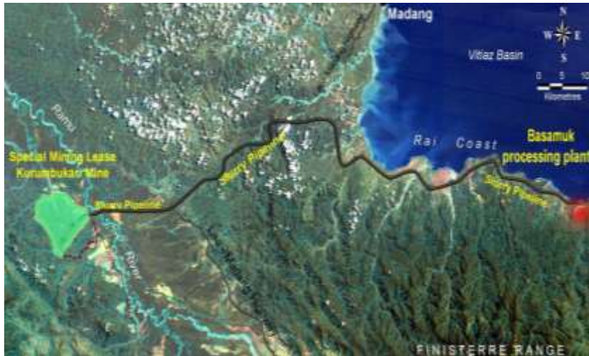
Figure 11 (From Ramu NiCo publicity video) shows the 135 km pipeline transporting slurry from the mine site to the processing plant. After crossing the Ramu River valley it follows the Lae Madang highway, before turning east near the coast and then proceeding to the processing plant.
