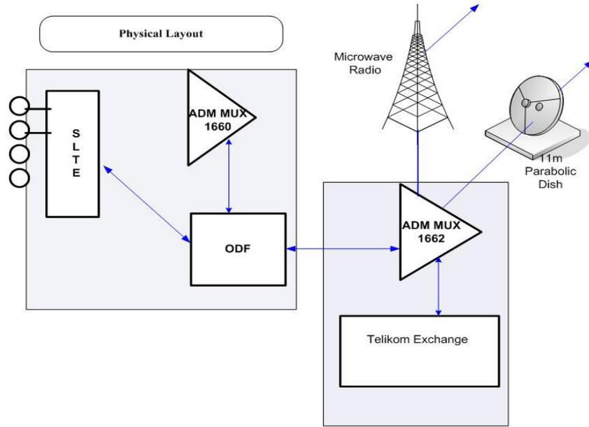
**Figure 11** The physical layout of the Cable Landing Station (CLS) at the Telkom Exchange premises in Madang is shown on the left, with main components, the Submarine Line Terminating Equipment (SLTE) and the Optical Distribution Frame (ODF). On the left, underground conduits bringing the fiber pair from BU4 via enter the building. The schematic building on the right is the PNG Telkom telephone exchange with its connection to the PNG domestic microwave line-of-sight and satellite backbone.
