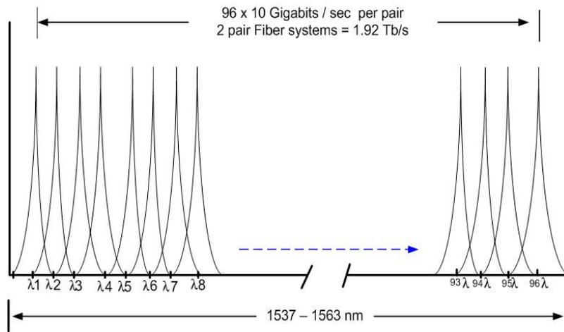
**Figure 3** illustrates lambda signal intensity distribution with DWDM as used by PPC-1<sup>20</sup>. On a single fiber pair 96 separate wavelengths (lambdas) or channels are tuned to slightly different frequencies in PPC-1 with each one capable of carrying 10 Gbps of data. The rapid drop off of signal intensity on either side of the carrier wavelength is designed to prevent cross talk between adjacent lambdas.
