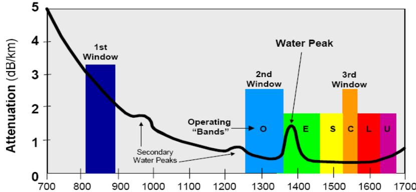
**Figure 2** The attenuation spectrum for optical fiber<sup>16</sup> shows bands of low IR absorption for single-mode fiber. These fibers usually operate in the 1310 nm (O band) or 1550 nm (S, G and L bands) regions, where attenuation reaches various minima.
