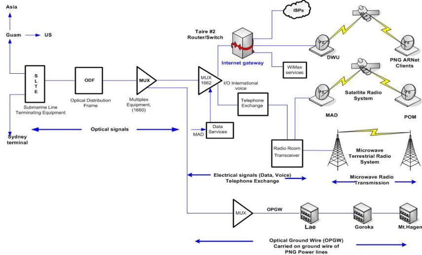
**Figure 12** Shows the components of the Cable Landing Station (LHS: SLTE, ODF and MUX) and then the many voice and data services which will benefit from the Madang PPC-1 connection. The options available from
