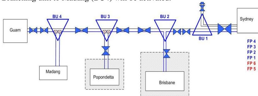
**Figure 5** is a logical diagram<sup>24</sup> showing how the schematic diagram in Figure 1 is implemented for PPC-1. with the present Branching Unit to Madang (BU4) and possible future branches to NZ (BU1), Brisbane (BU2), Port Moresby or Popondetta (BU3). Two fiber pairs are for present implementation, with an additional 4 pairs available to install spurs to further strategic locations.
