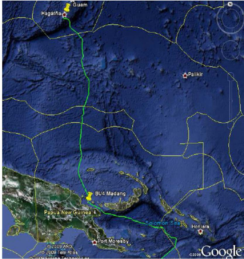
**Figure 7** Northern portion of the 6900 km PPC-1 submarine cable<sup>28</sup> showing the Madang BU4 passing through Vitiāz Strait parallel to the Finisterre Range, skirting Astrolabe Bay before veering north and traversing deep ocean trenches on its way to Guam.
