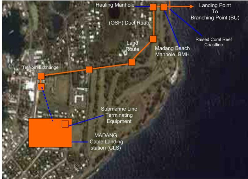
**Figure 10** Superimposed on satellite imagery is the PPC-1 landing point on the Madang coast beside the iconic Coast Watchers Lighthouse. After passing through the Beach Manhole, the cable passes through a series of Hauling Manholes before reaching the CLS situated on the PNG Telikom Exchange premises at Modilon.
