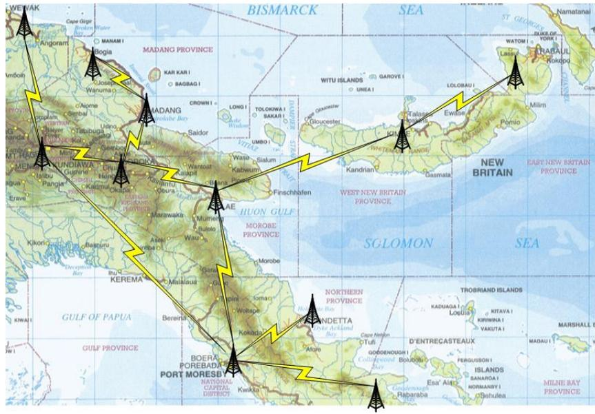
**Figure 9** Important sectors of the PNG internal domestic telecommunications trunk network<sup>30</sup> initially constructed to allow important centres to take advantage of the SEACOM cable. The network uses line-of-sight microwave (5-7 GHz) services involving chains of repeater stations located on mountain peaks every 50 km. The proposed fiber optic backbone will use PNG Power transmission lines as bearers and will follow the road system. Shown are the main transmitter mast locations.
