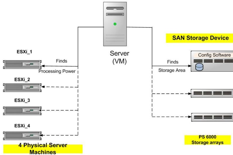
**Figure 11 Processing power and storage for each VM**
