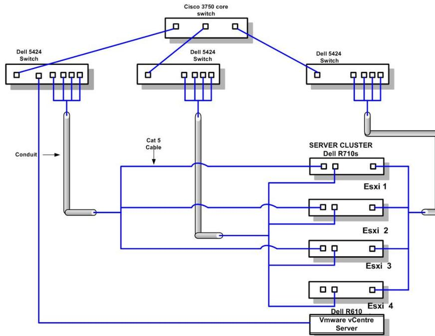
**Figure 5 DWU Data Centre server Ethernet connections**
