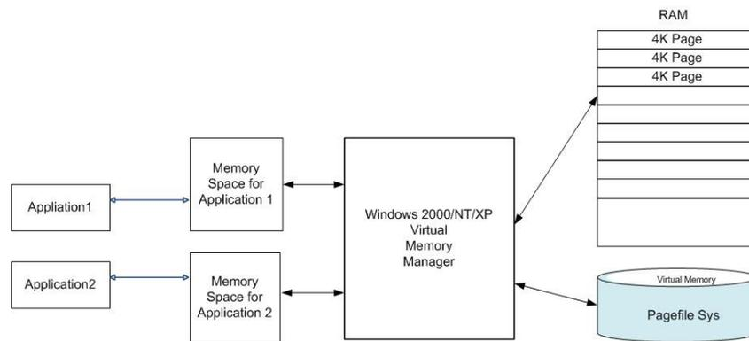
**Figure 1 Decoupling by a VMM**
