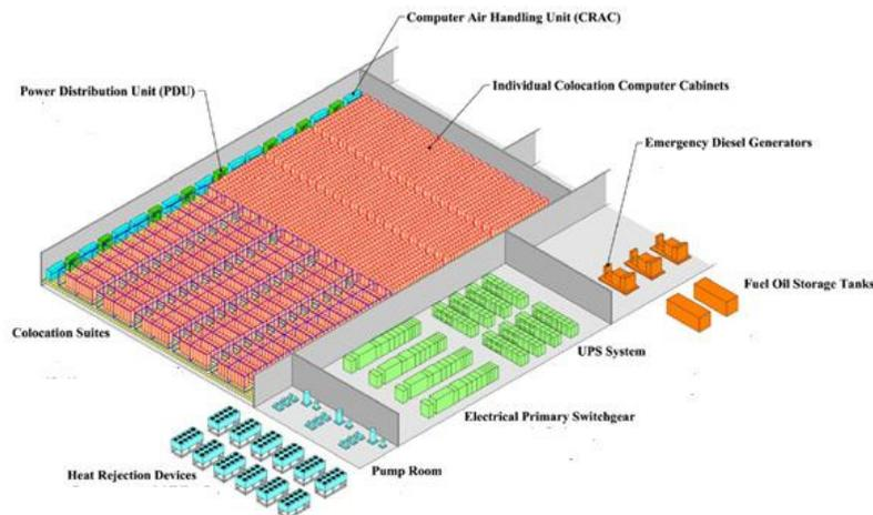
**Figure 16 Main components of a cloud computing data center**
