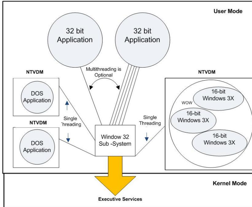
**Figure 2 Traditional applications of virtual machines**
