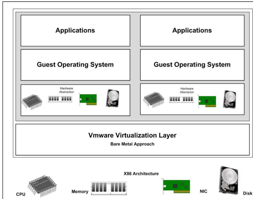
**Figure 3 Bare metal approach to hardware virtualisation.**
