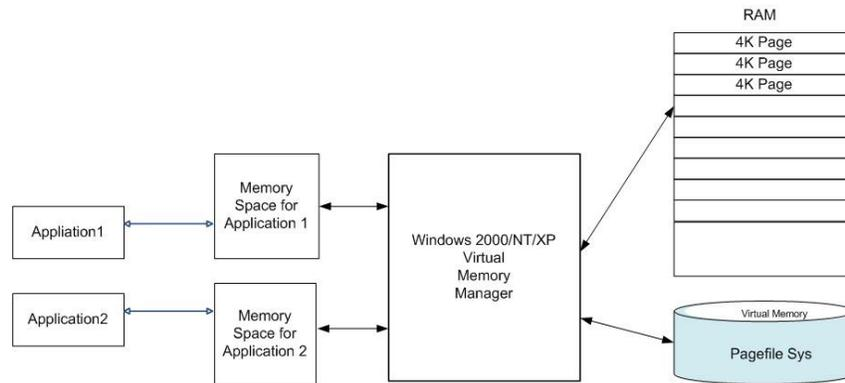
**Figure 1 Decoupling by a VMM**
