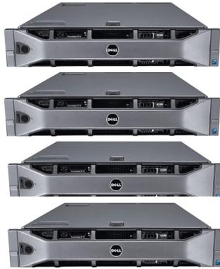
**Figure 4 Four clustered rack mounted physical servers**
