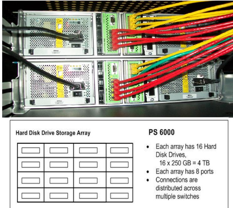
**Figure 10 SAN physical connections**
