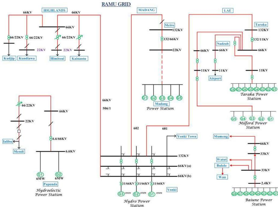
**Figure 3:** Simplified single line schematic diagram of Ramu Grid showing transmission lines (red) and bus lines (black)
