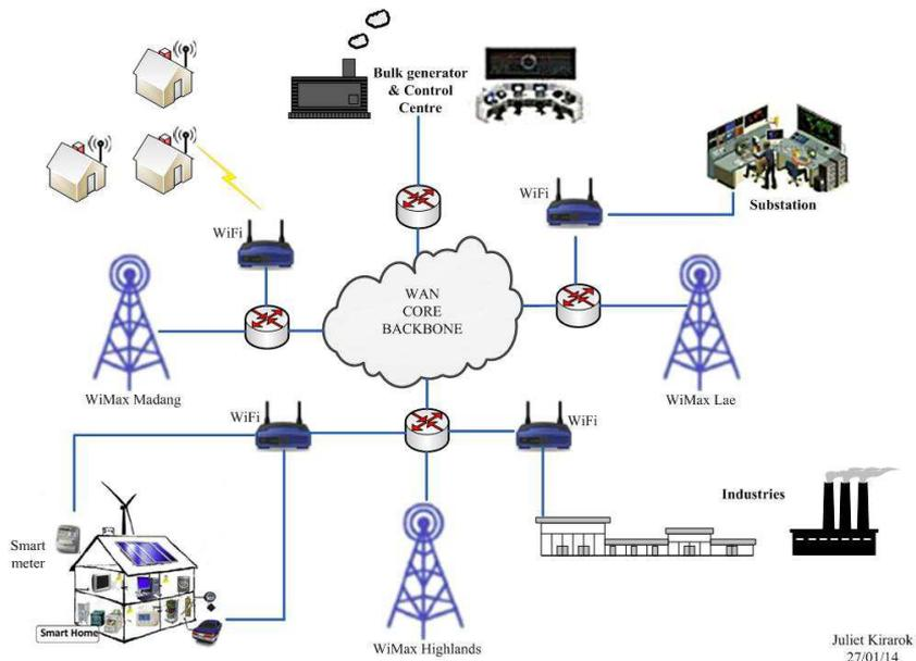
**Figure 8:** Schematic diagram showing a hypothetical wireless sensor and actor network for the Ramu grid
