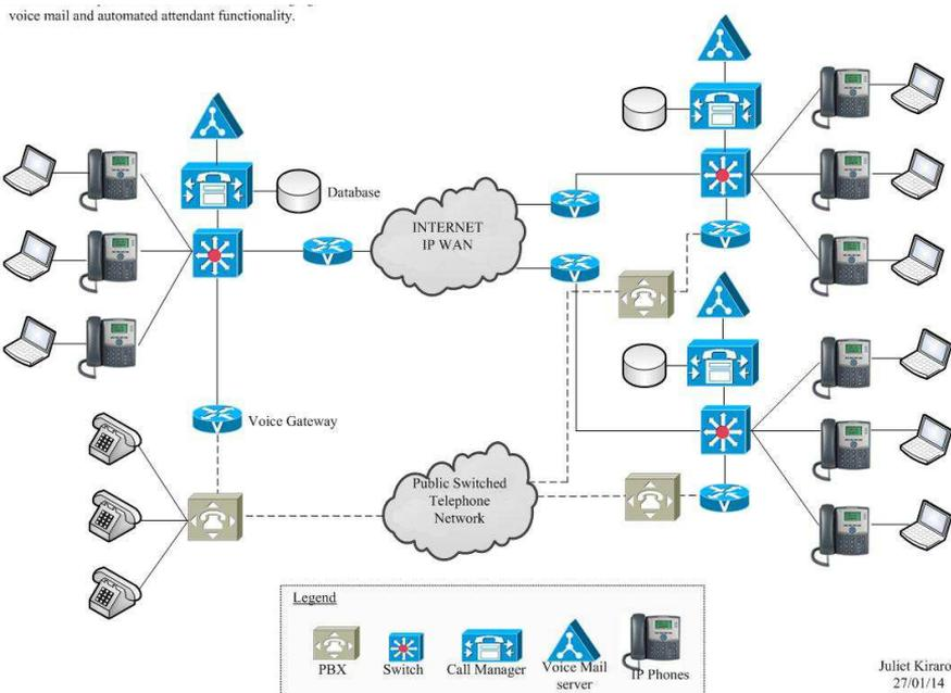
**Figure 9:** Logical diagram showing the IP based end-devices with Internet IP WAN connectivity as a telecommunication network alternative to the PSTN
