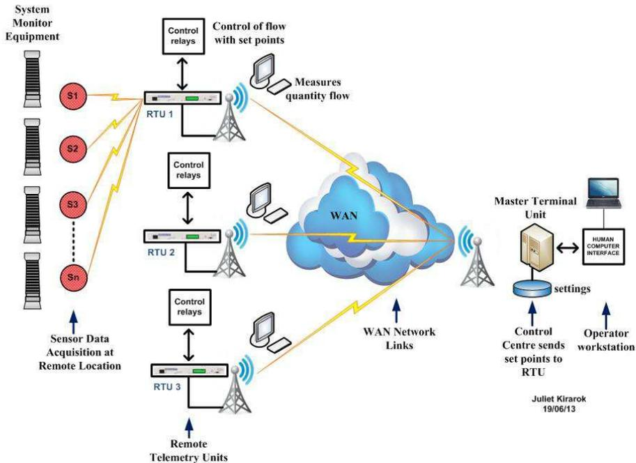
**Figure 6:** SCADA system components coordinating a network of error detecting intelligent devices using a point to multipoint configuration
