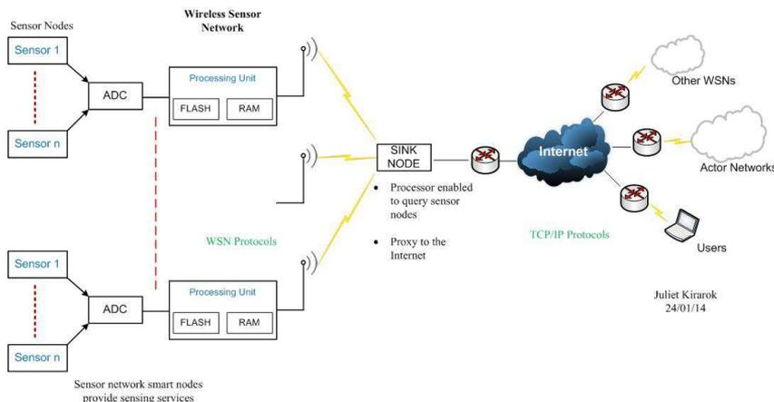
**Figure 7:** Wireless Sensor and Actor Network to enable the electricity grid to function as what is now known as a Smart Grid
