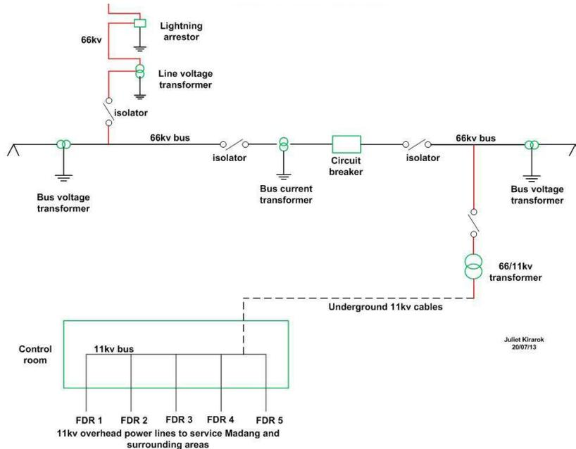
**Figure 4:** Single Line schematic diagram for the Meiro Distribution Substation, Madang
