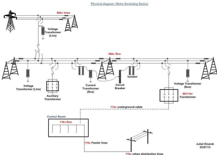
**Figure 5:** Three phase physical diagram for Meiro Distribution Substation, Madang
