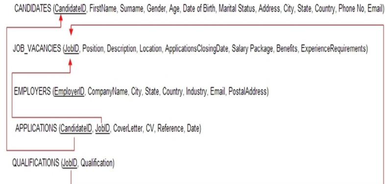
Figure 3 The relational schema which transforms the entity relationship diagram into an implementation model, thus indicating primary to foreign key relationships that would exist in the physical tables when implemented.
