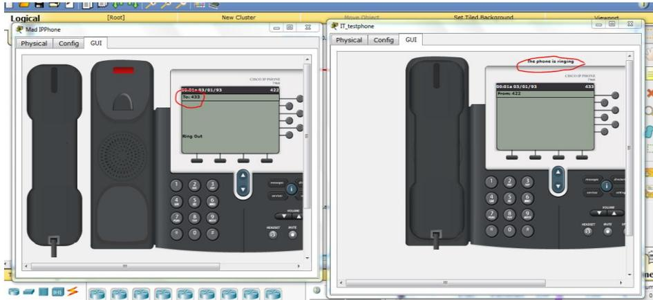
**Figure 12.** Once the ip phones are configured correctly, they should automatically receive dial numbers assigned.
