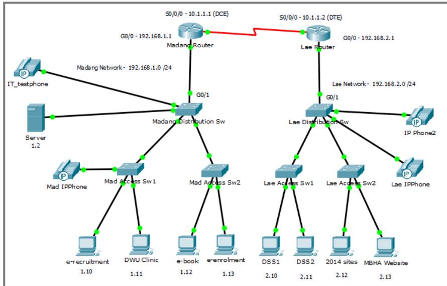
**Figure 11** An overview of the small-medium business network design modelled inside Packet Tracer
