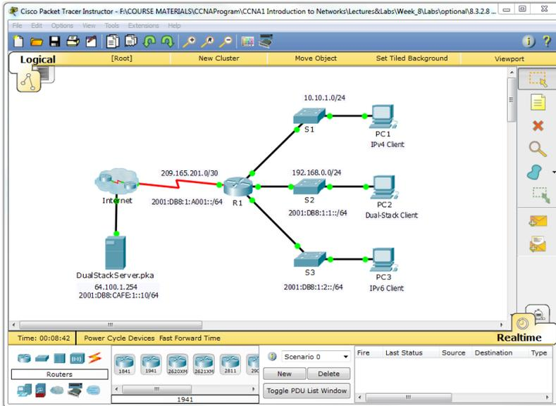
**Figure 2.** A sample PT window showing simulated networking network topology in the workspace with various devices, derived from the selection pane, now available for configuration by simply clicking on the appropriate icon.
