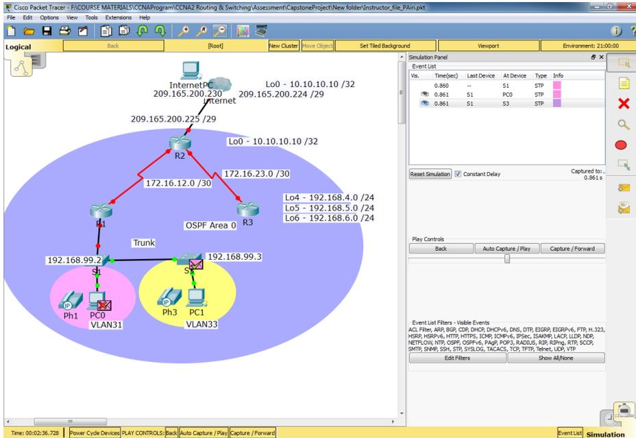
**Figure 6.** Simulation mode is illustrated in this figure. A basic packet can be sent from any sender device to destination and the route the packet takes can be observed in PT.
