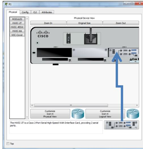
**Figure 7.** A module is selected and then inserted into the device.
