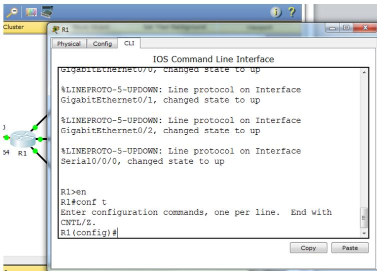
**Figure 3.** Command Line Interface (CLI) tab where IOS of a switch or router can be accessed and commands entered.
