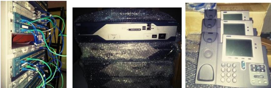
**Figure 1.** The initial 12-unit equipment rack on the left, with a new router (centre) and Voice over IP phones (VOIP) (right) as additional equipment for student laboratory work simulating real works situations.
