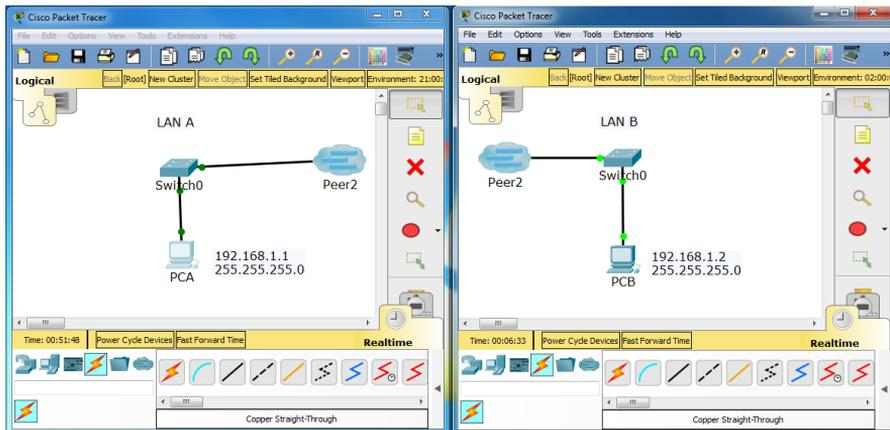
**Figure 8.** The multiuser functionality in Packet Tracer enables multiple networks on different computers to interact.
