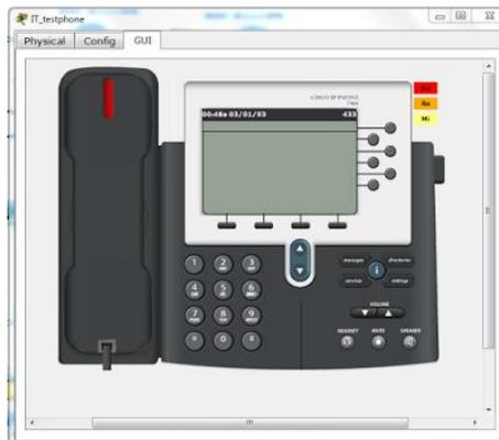
Once all the tasks are completed, the student now has to verify by dialing 422 and checking if IP phone 1 correctly receives the call. The software can simulate picking up the handset to answer the call.
